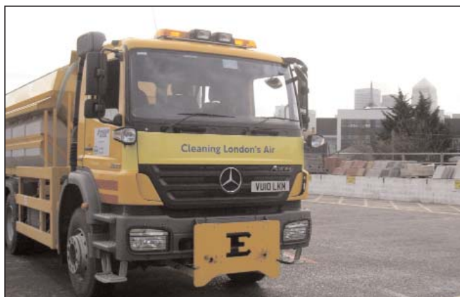
A converted gritter will be used to spread the CMA suppressant
